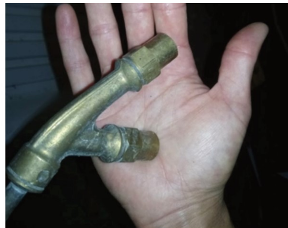
Figure 15: (A) REC 15 AC1 electric driven hand sprayer by Birchmeier; (B) Y-form double nozzle
